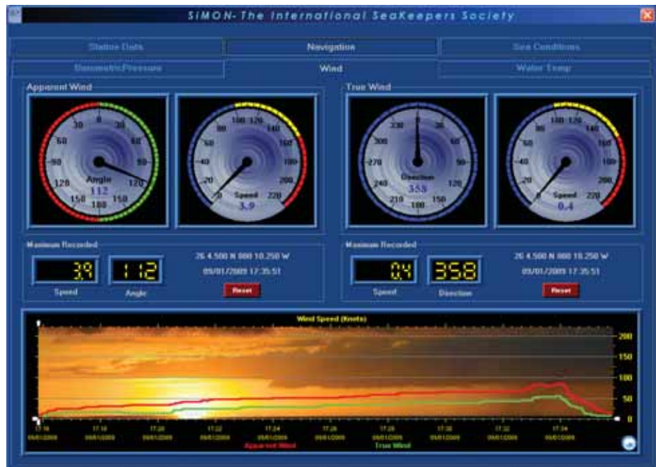
The screen above shows the Actual Wind and True Wind speeds, along with angle and direction information. Other screens can be accessed for current data on Barometric Pressure, Humidity, Air Temperature, etc.
