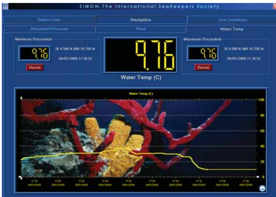
The screen above shows the real-time near surface Water Temperature, along with the minimum and maximum temperatures recorded for the period set. Other oceanographic measurements such as Salinity, pH, Chlorophyll, etc. are accessed on other screens.
