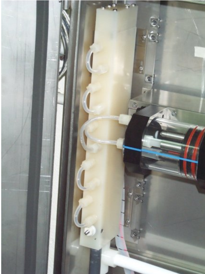
Figure 6.2 Manifold and sensor connections
