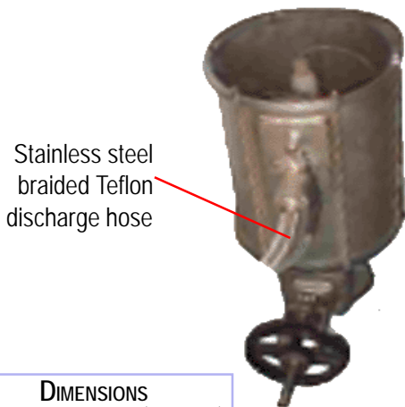
Containment vessel with emergency shut off solenoid valve
