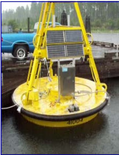
NOAA/NDBC 3 meter buoy equipped with low power instrument box
