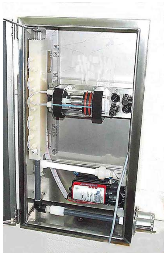
Figure 2. Photograph illustrates a sensor module plumbed into the distribution manifold in the SeaKeeper 1000.
