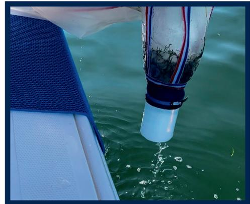
*Sample collection undergoing filtration from a Neuston Net tow.*
