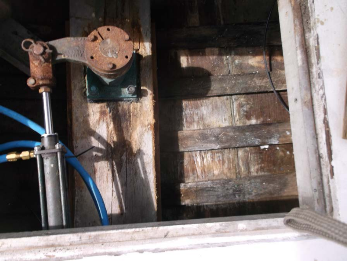
Photo No. 9 Aft bilge planking in good condition.
