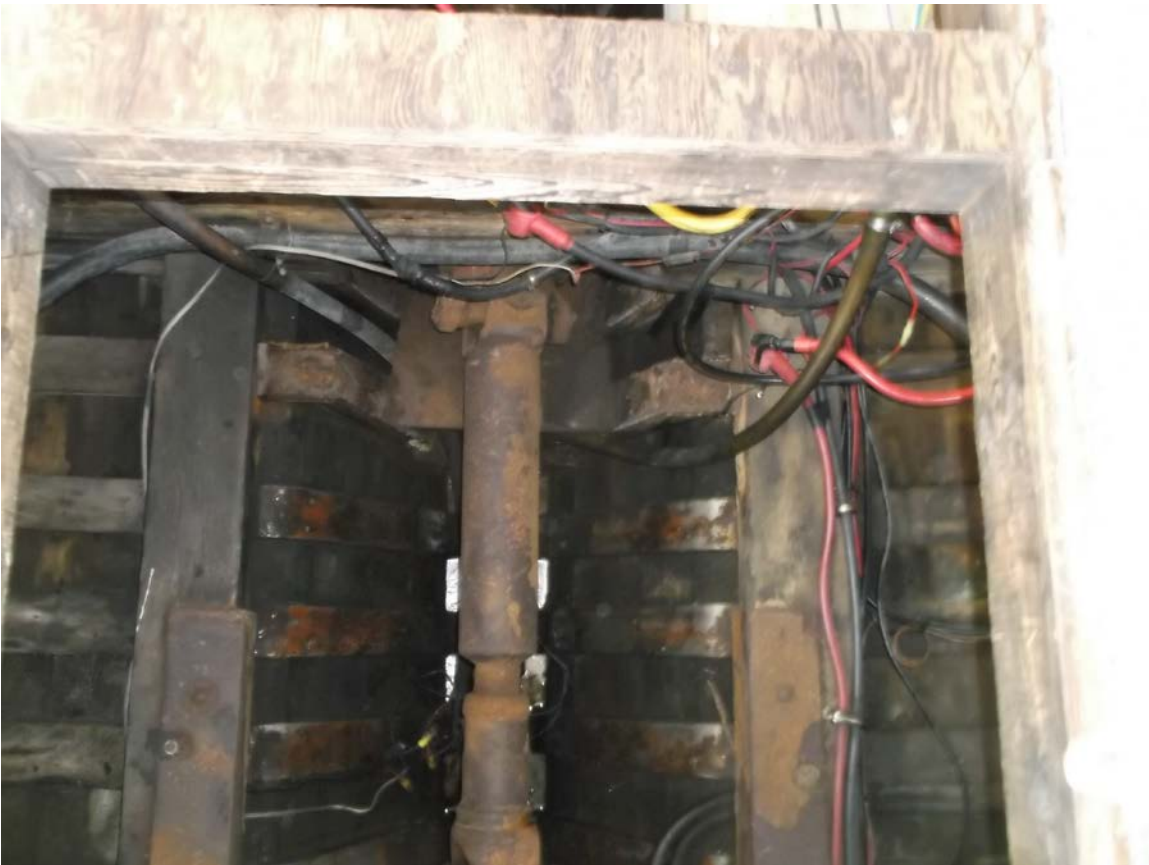
Photo No. 8 Bilges amidships are practically dry and clean.
