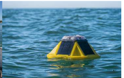
The Spotter ocean sensor by SoFar, is deployed while the vessels are underway to their next destinations.
